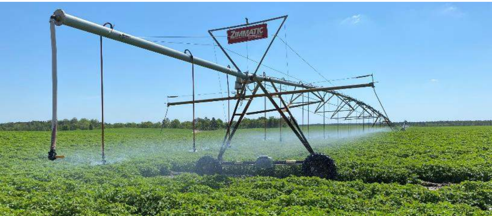
Figure 2-16. Center pivot - fixed rate irrigation system with best nozzle technology in use at Walther Farms, April 2021.
