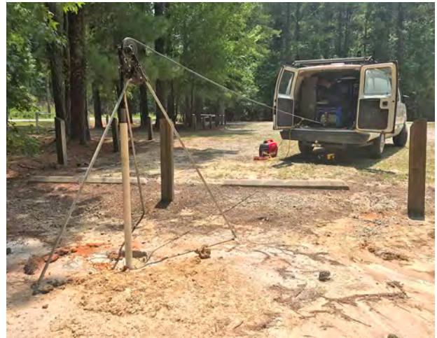
Figure 29. Collecting a gamma-ray log through the 2-inch PVC casing of the new shallow well LEX-1703 at the Congaree Creek Heritage Preserve in Lexington County.
