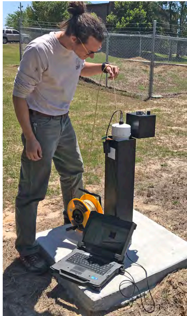
Figure 5. Manual measurement of a water level using an electric tape.
