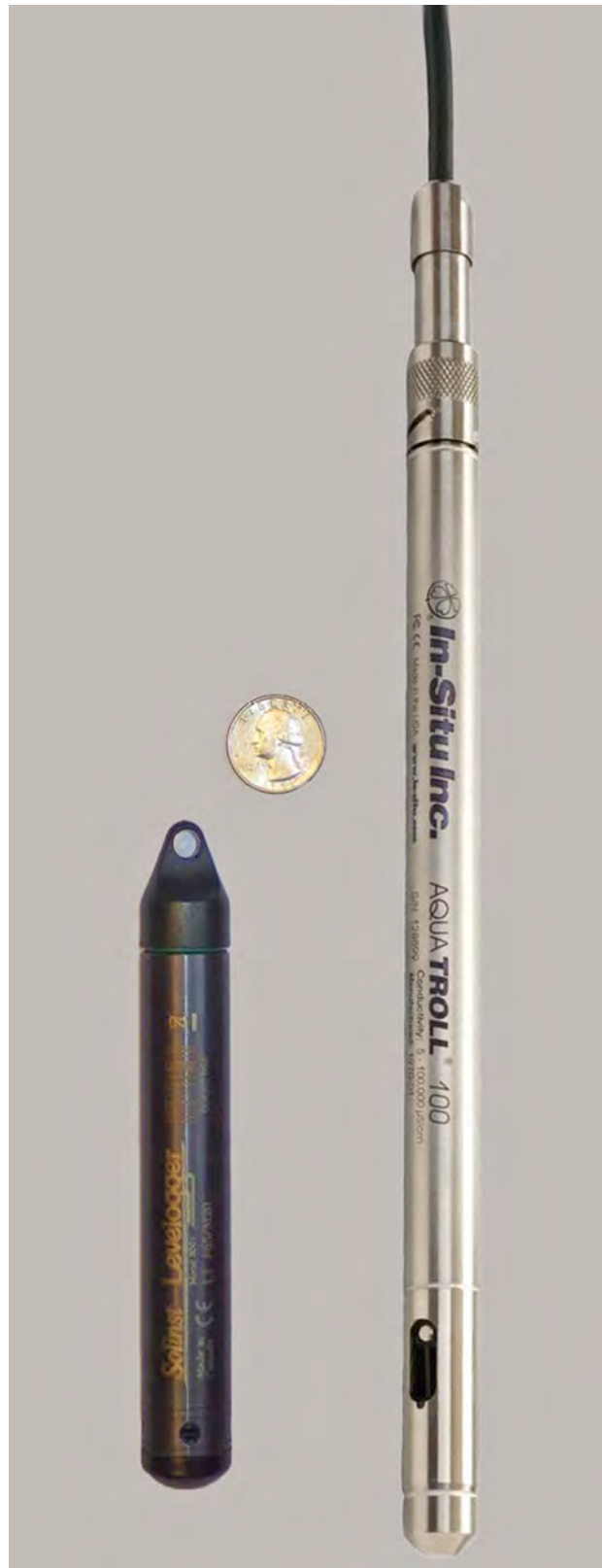
Figure 7. Two types of automated data recorders used in the SCDNR network: Solinst® Levelogger® (left) measures water-level; In-Situ® Aqua TROLL® (right) measures conductivity and temperature.
