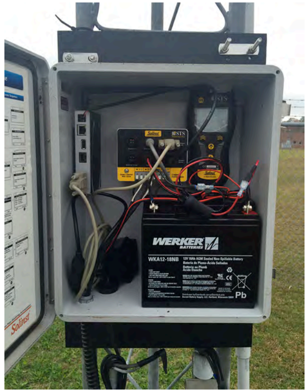
Figure 16. 9100 STS Gold Telemetry system manufactured by Solinst Canada Ltd.
