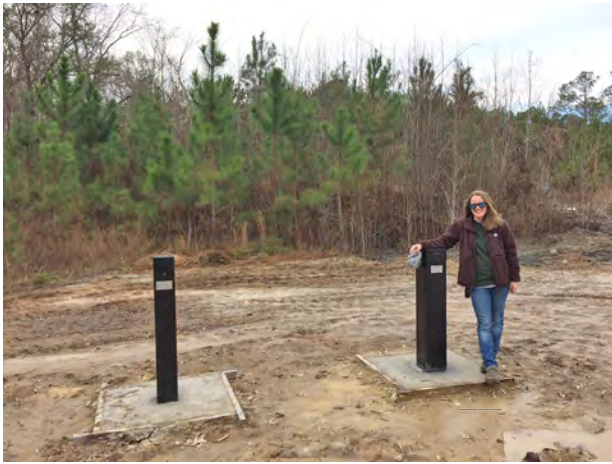
Figure 26. Two new monitoring wells at 8 Oaks Park in Georgetown County. GEO-0390 (right) is a 4-inch well, 640 feet deep and screened in the Crouch Branch aquifer. GEO-0391 (left) is one of the 10 monitoring wells drilled in late 2018 and early 2019 to monitor the surficial aquifer system throughout the Coastal Plain.
