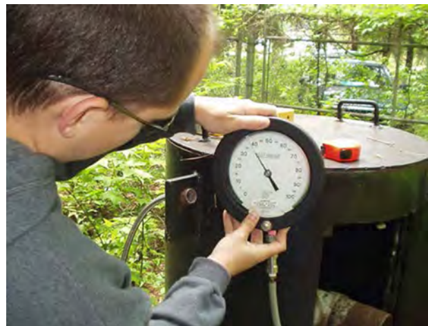
Figure 6. Manual measurement of a water level in a flowing well using a pressure test gage.
