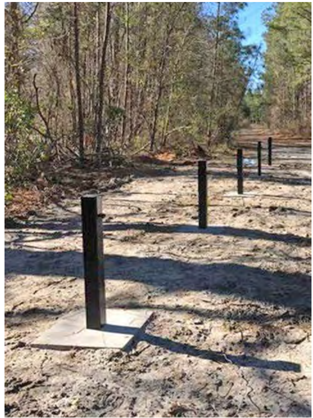
Figure 23. The five monitoring wells that make up the Sumter cluster site at the Central Carolina Technical College Natural Resources Center.
