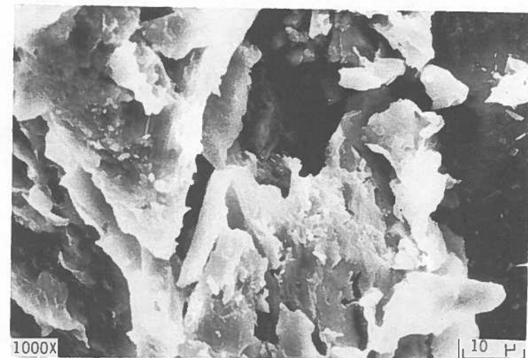
Figure 7. Photomicrograph from SEM analysis of 1,222-ft bls sample, showing coarse- to fine-grained sand (a), authogenic kaolinite (b), and feldspar dissolution (c) (clockwise from upper left).
