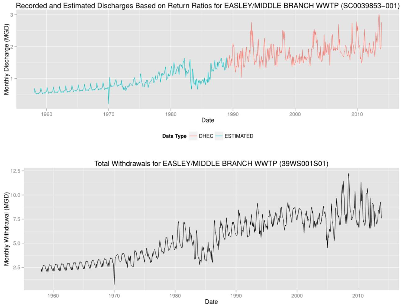
**Figure 4.2: (TOP) DHEC Provided and Estimated Monthly Discharge. (BOTTOM) Monthly Withdrawals Used for Hindcasting**
