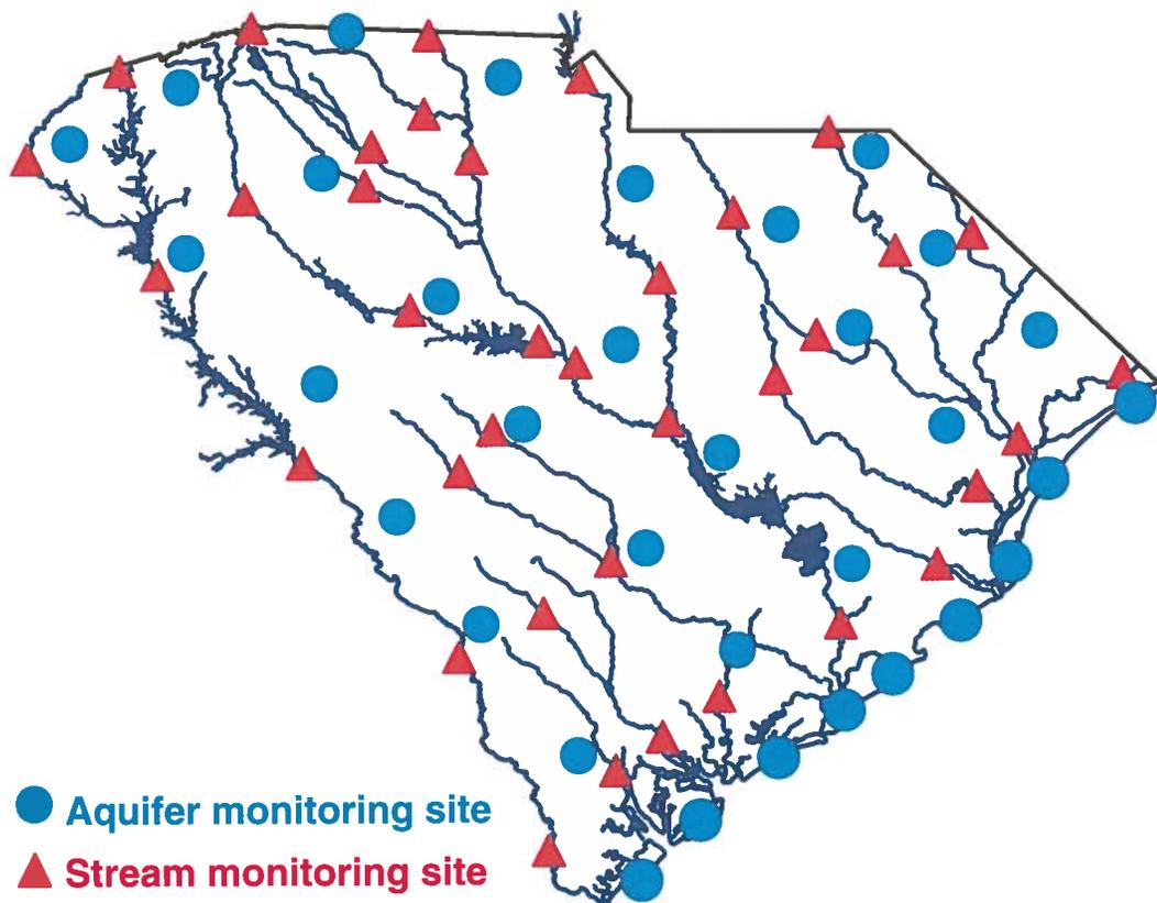
Figure 25. Basic network for monitoring quantity and quality of water in streams, lakes, and aquifers of the State.
