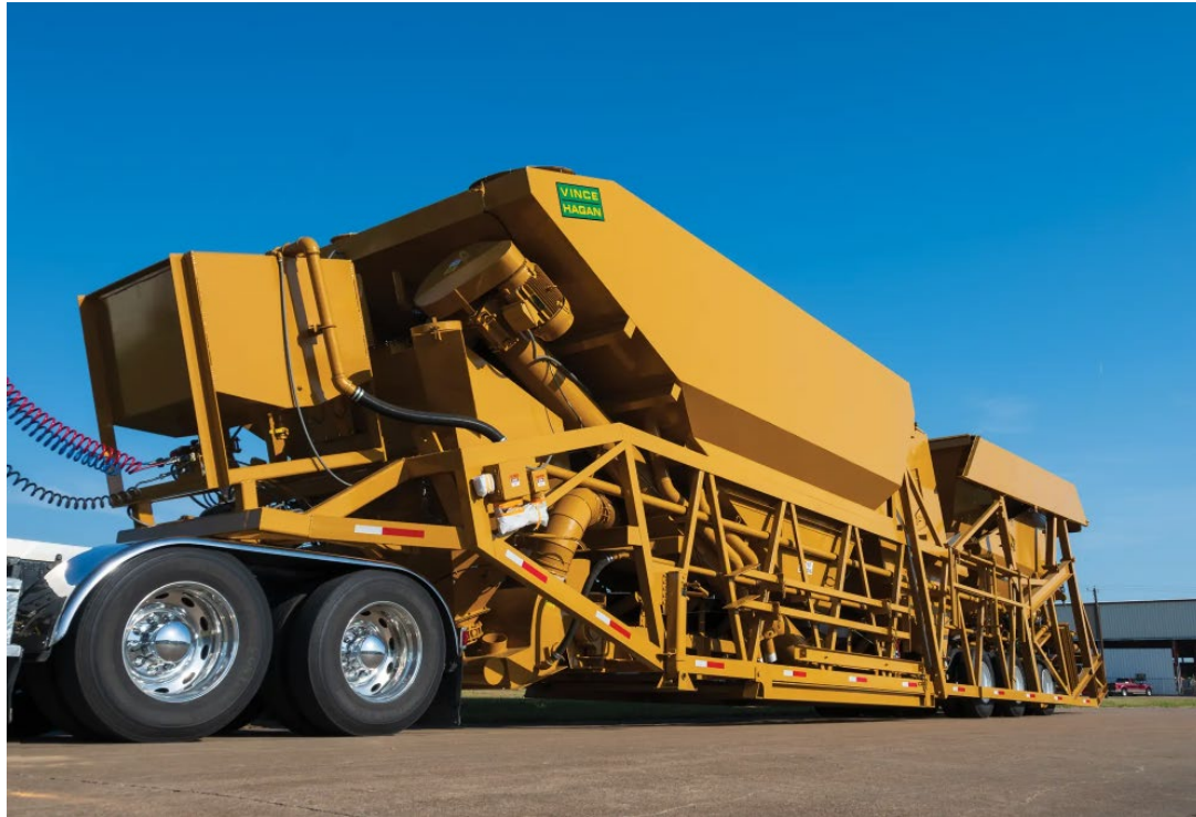
Portable Concrete Plant
