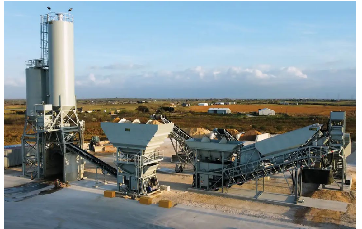
Stationary Concrete Plant
