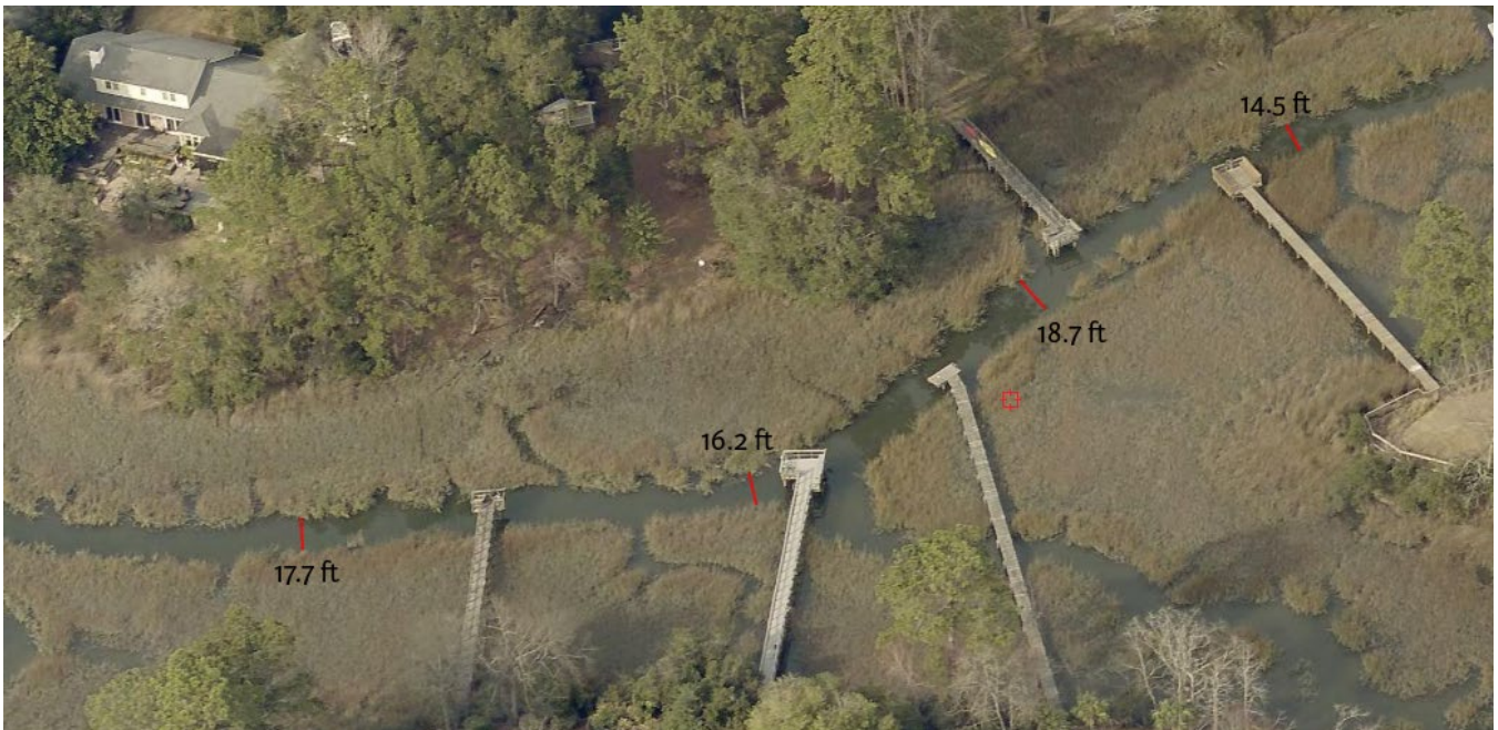
Figures 1 and 2: Examples of navigation and public access limitations with docks on small creeks.
