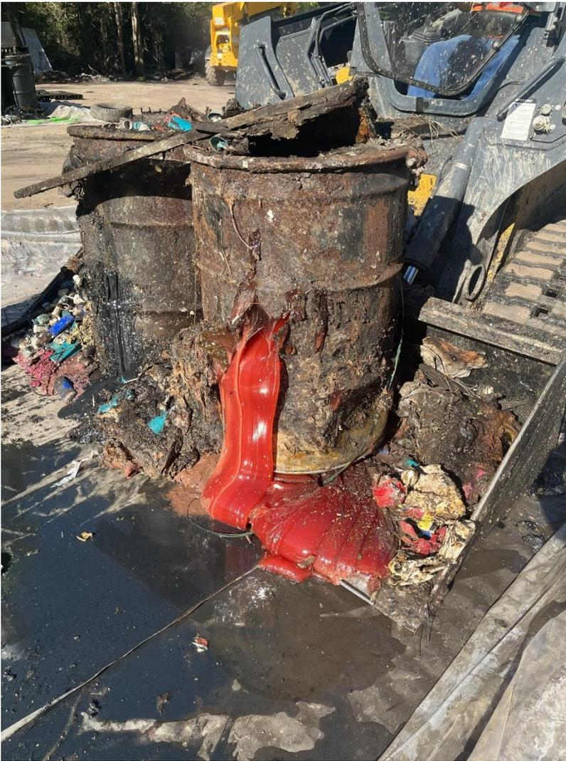
*Polymer leaking out of a heavily damaged container at the Trebie Road Site in FY2023.*
