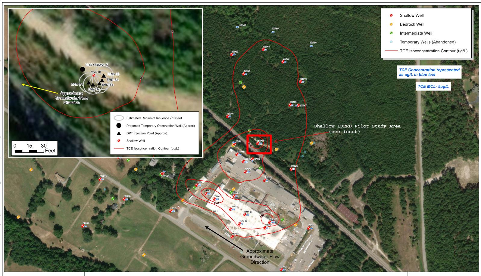
101 Research Drive Columbia, SC 29203-9389 T: (803) 254-4400 F: (803) 771-6676 Figure 3 : Enhanced Reductive Dechlorination (ISB and ISCR) Pilot Study Area - Shallow Zone Shakespeare Composition Structures
