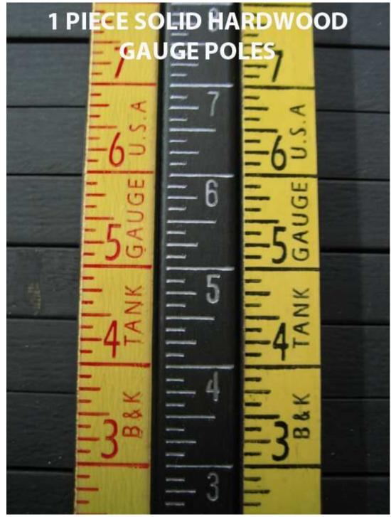
Typical gauging stick used in conjuction with tank chart to determine the volume of fluid in tank.
