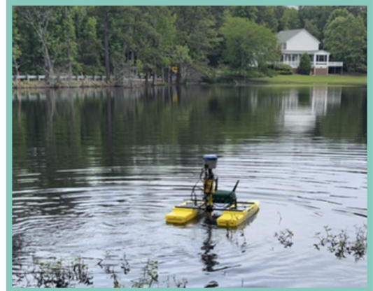
The autonomous boat used for performing bathymetric surveys.
