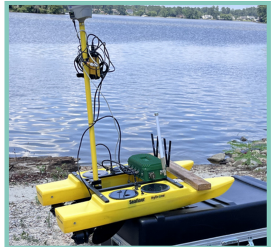
The autonomous boat used for performing bathymetric surveys.
