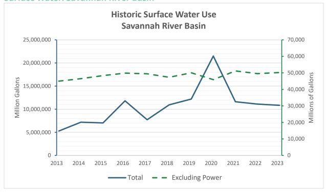
Figure 57: Historic Surface Water Use in the Savannah River Basin, 2013 – 2023. Please note the left axis corresponds to the total water use (blue line), while the right axis corresponds to the water use without power production (green).\*2015 to present saw an increased use for hydroelectric power users, including the installation of 3 new power plants. Also, 2020 saw increased hydropower use due to a large volume of water released through the lake system.
