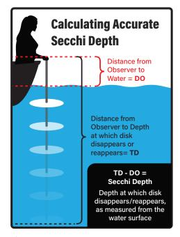
**Figure 22.** Official depth should be measured from water surface to the disk, NOT from where you are holding the measuring tape.
