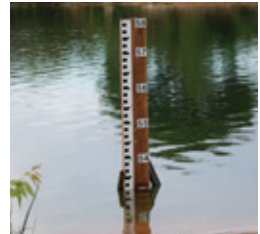
Figure 23. Lake level gauge
