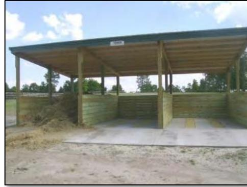
Figure 16. Example of Large Composter for Waste Management
