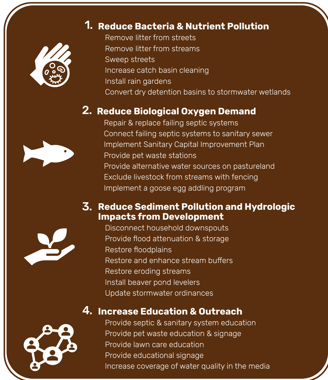
Figure 5.1 Diagram of watershed objectives & management measures
