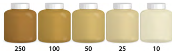
Figure 2.13 These bottles show various turbidity levels measured in NTU (The Laboratory People, 2021)
