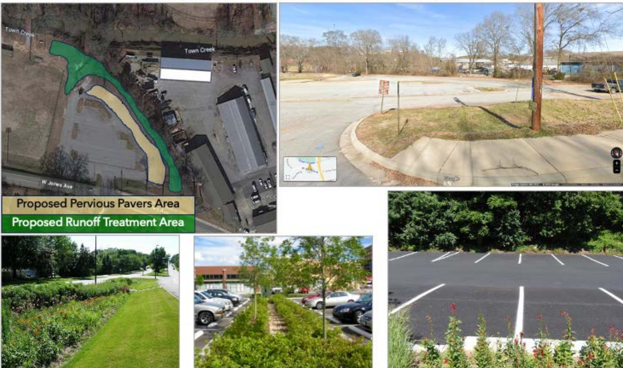
Fig. 41. Overview of large parking area's opportunities for stormwater treatment and retention (top left); street view of existing parking area (top right); example of porous asphalt use in a parking lot with center drainage and no curbs (bottom right); example of curbless planted parking lot median with drainage from Pennsylvania State University Sea Grant (bottom middle); example of bioretention treatment area with curb cut from RK&K (bottom left)
