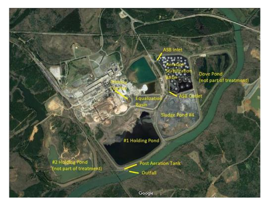
Figure 4-1 Wastewater Treatment Configuration
