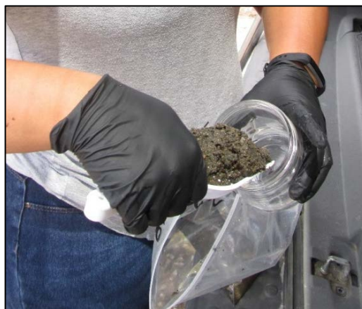
Sediment is measured out to be tested for non-radiological parameters
