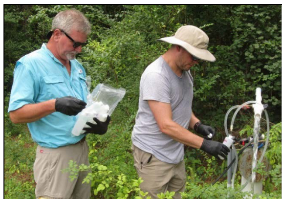
Collecting water from pump to test for non-radiological material
