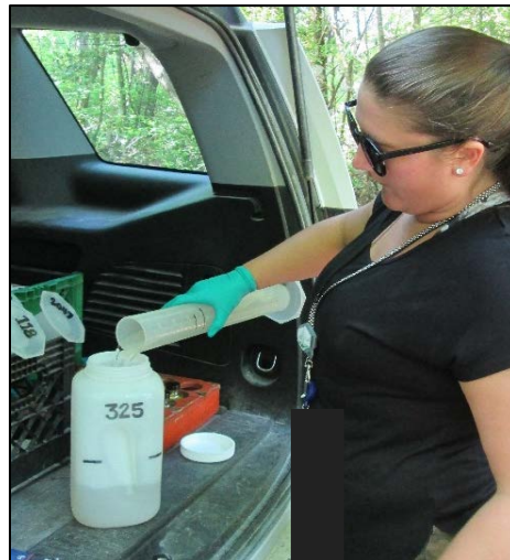
Pouring a monthly composite sample to be tested for gamma and gross alpha/beta radionuclides
