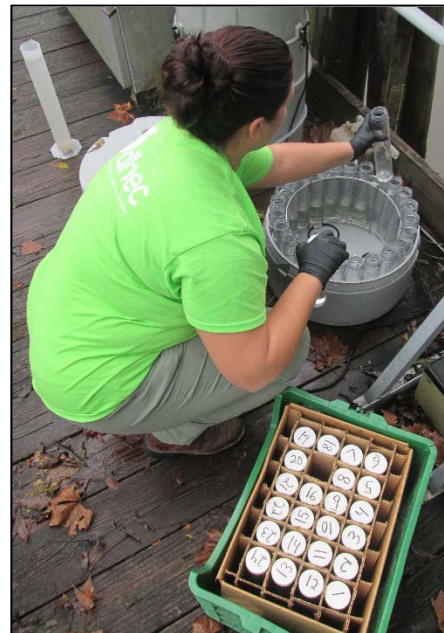
Collecting samples to be tested for tritium using the early detection system at SV-118
