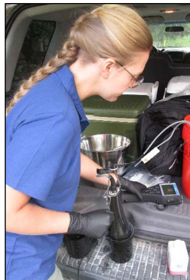
Standardizing the Horiba Water Testing System
