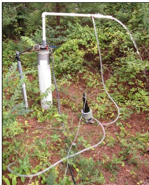
Above: Cluster well being pumped and field tested for field parameters.
