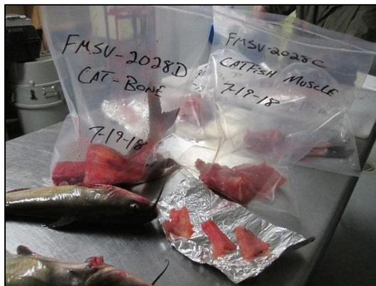
Individual fish parts are combined to form composite samples which are tested for strontium (bones) and gamma and metals (muscles)
