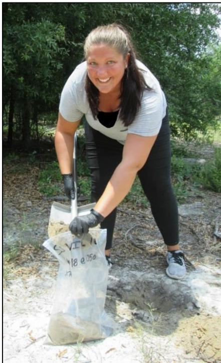
Collecting soil samples which will be tested for radiological material and metals
