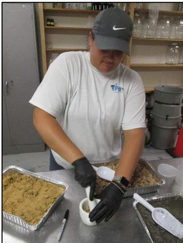
Dried samples are pulverized before being sent to the Columbia lab to be analyzed for radionuclides
