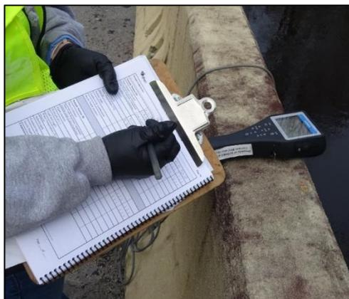
Recording field parameters: DO, pH, temperature, conductivity, and total dissolved solids
