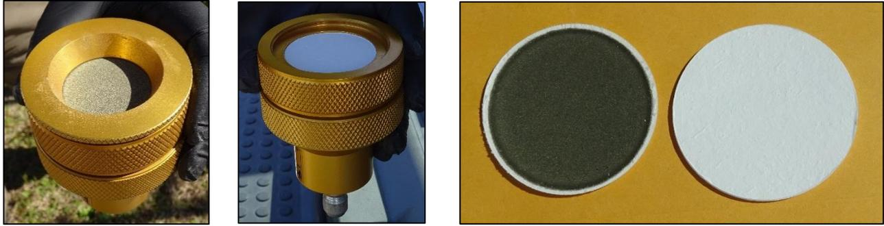
Glass fiber filter being collected for total suspended particulates: Used filter (left) vs. unused filter (right)
