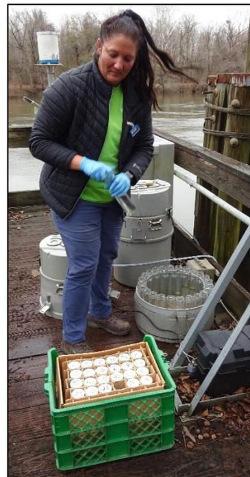
Collecting samples to be tested for tritium using the early detection system at SV-118
