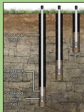
**NETWORK WELLS** are single wells at a specific location screened in a specific aquifer.
