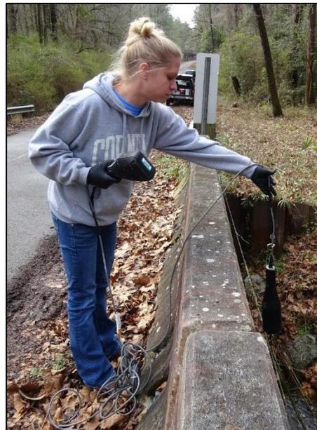
Using a Horiba Water Quality Meter to determine field parameters
