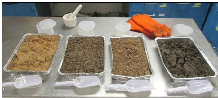
Sediment samples after being placed in drying oven
