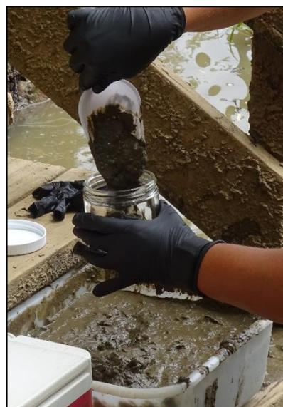
Sediment is measured out to be tested for non-radiological parameters
