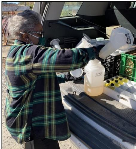
Pouring off a composite sample to be used for monthly alpha, beta, and gamma analysis
