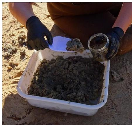
Preparing sample for non-radionuclide lab analysis
