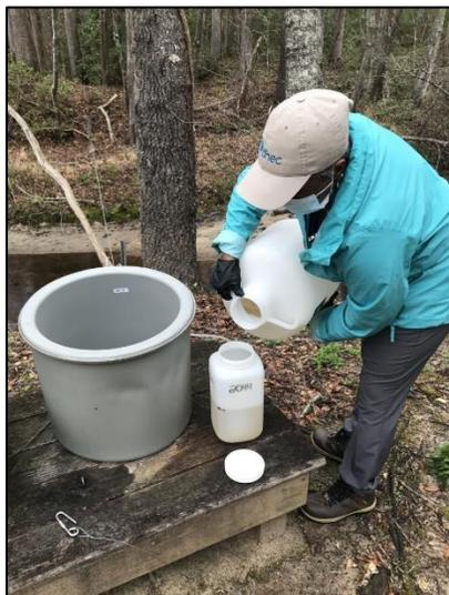
Pouring a sample to be tested for gamma-emitting radionuclides
