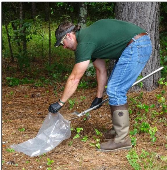
Collecting soil samples which will be analyzed for radiological material and metals
