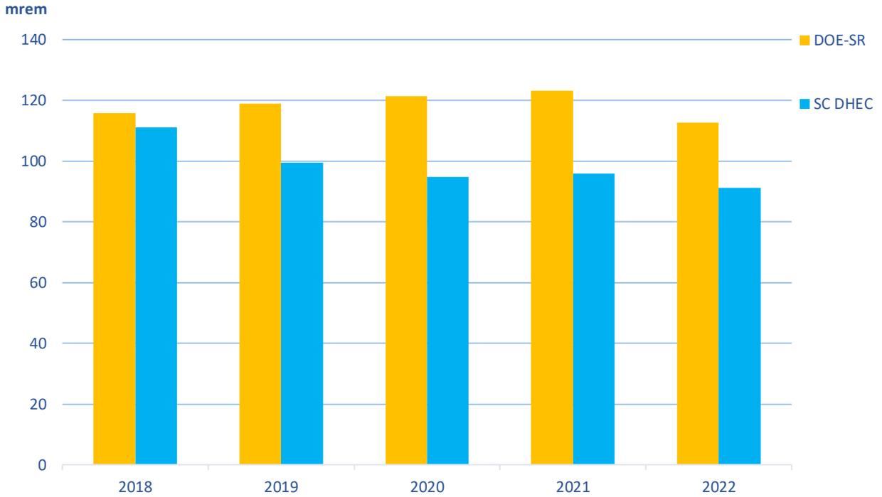
Figure 4. DOE-SR and DHEC Comparison of Average Tritium in Air at the SRS Perimeter (SRNS, 2019-2023; DHEC, 2020a-2022a)
