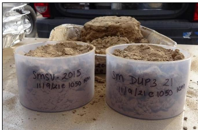
Prepped samples being sent to the lab for radionuclide analysis
