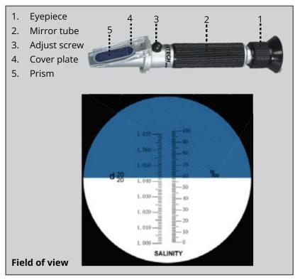
Parts of a refractometer.
