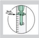
Read the syringe from the bottom of the green ring. In this example, the result is 4.0 mg/L or ppm.
