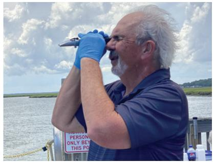
Using a refractometer to measure salinity.
