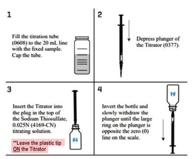
NOTE: If small air bubbles appear in the titrator barrel, expel them by partially filling the barrel and pumping the titration solution back into the reagent container. Repeat until bubble disappears.
