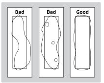
Liquid should completely cover the prism with no air bubbles.
