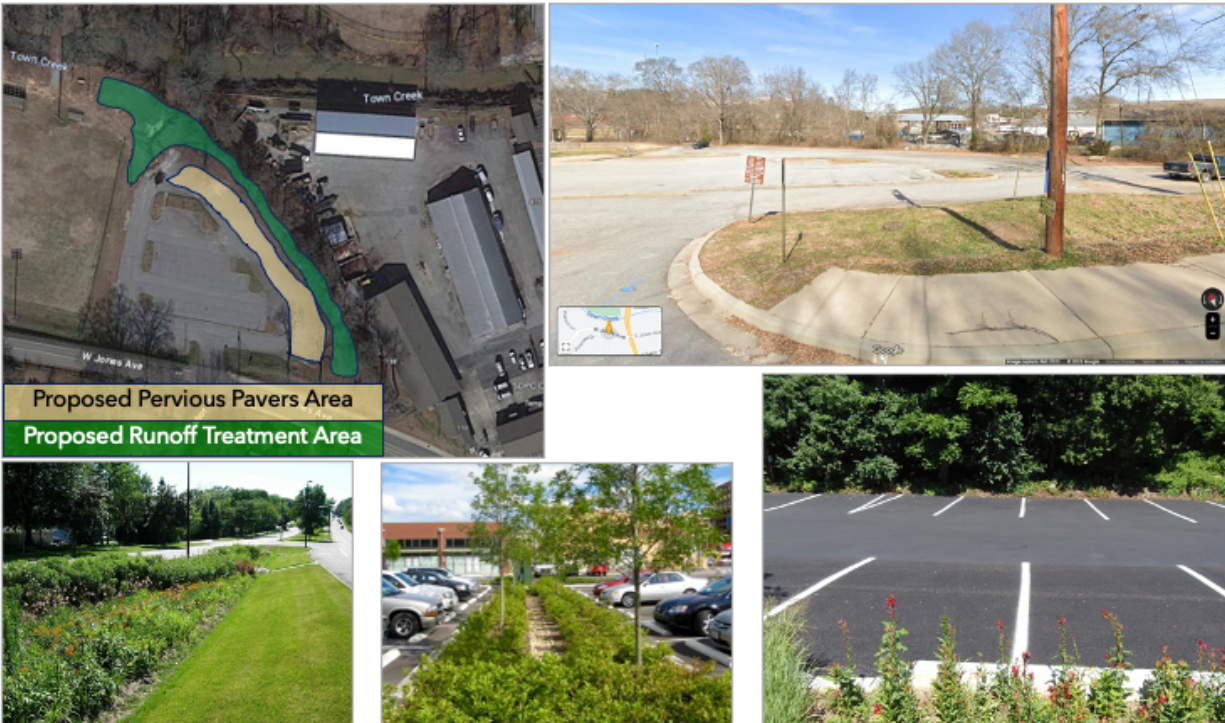
Fig. 41. Overview of large parking area's opportunities for stormwater treatment and retention (top left); street view of existing parking area (top right); example of porous asphalt use in a parking lot with center drainage and no curbs (bottom right); example of curbless planted parking lot median with drainage from Pennsylvania State University Sea Grant (bottom middle); example of bioretention treatment area with curb cut from RK&K (bottom left)
