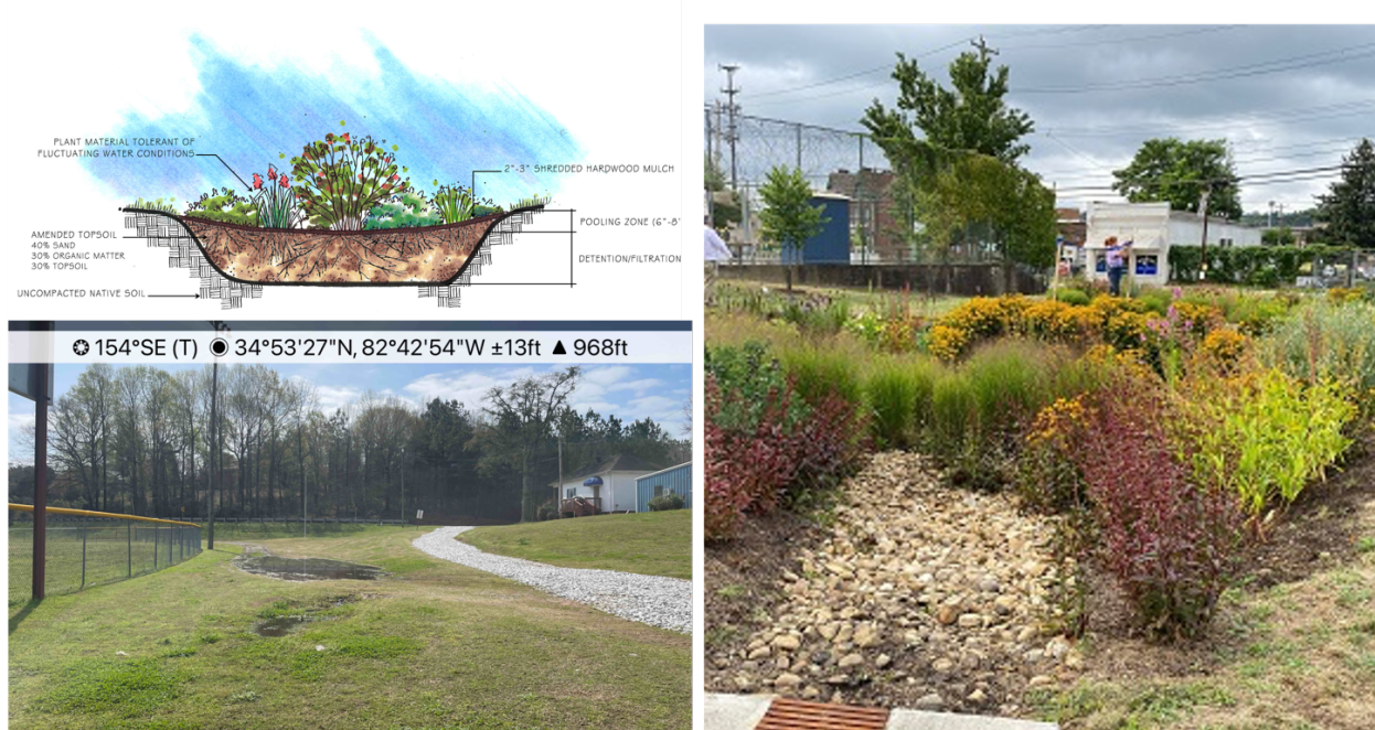
Fig. 39. The creation of a bioswale in this already pooling, low-lying area would provide beautification, stormwater treatment, and be an ideal location for education. Photo credits: Clemson Extension Carolina Clear Rain Garden illustration (top left), bioretention basin photo from Western Pennsylvania Conservancy (right), low-lying area at Jaycee Park (bottom left).
