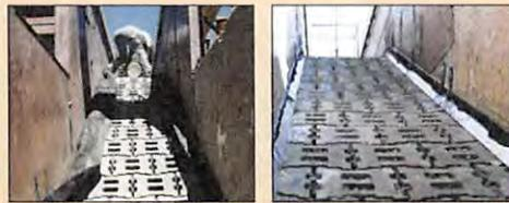
SHOREBLOCK® SD has been successfully tested by Colorado State University, in accordance with the hydraulic performance testing protocol established by the U.S. Federal Highway Administration. (FHWA-RD-89-199).
