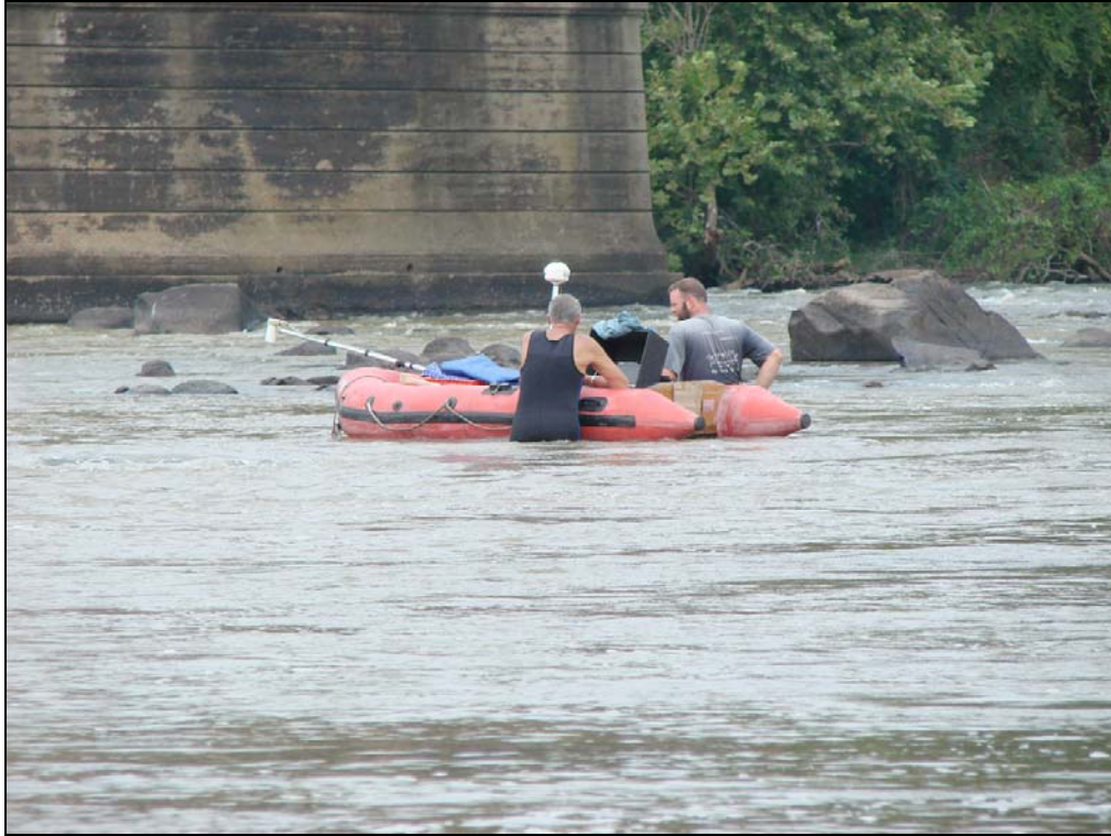
3. Performing geophysical survey via wading with equipment contained in a rubber raft.
