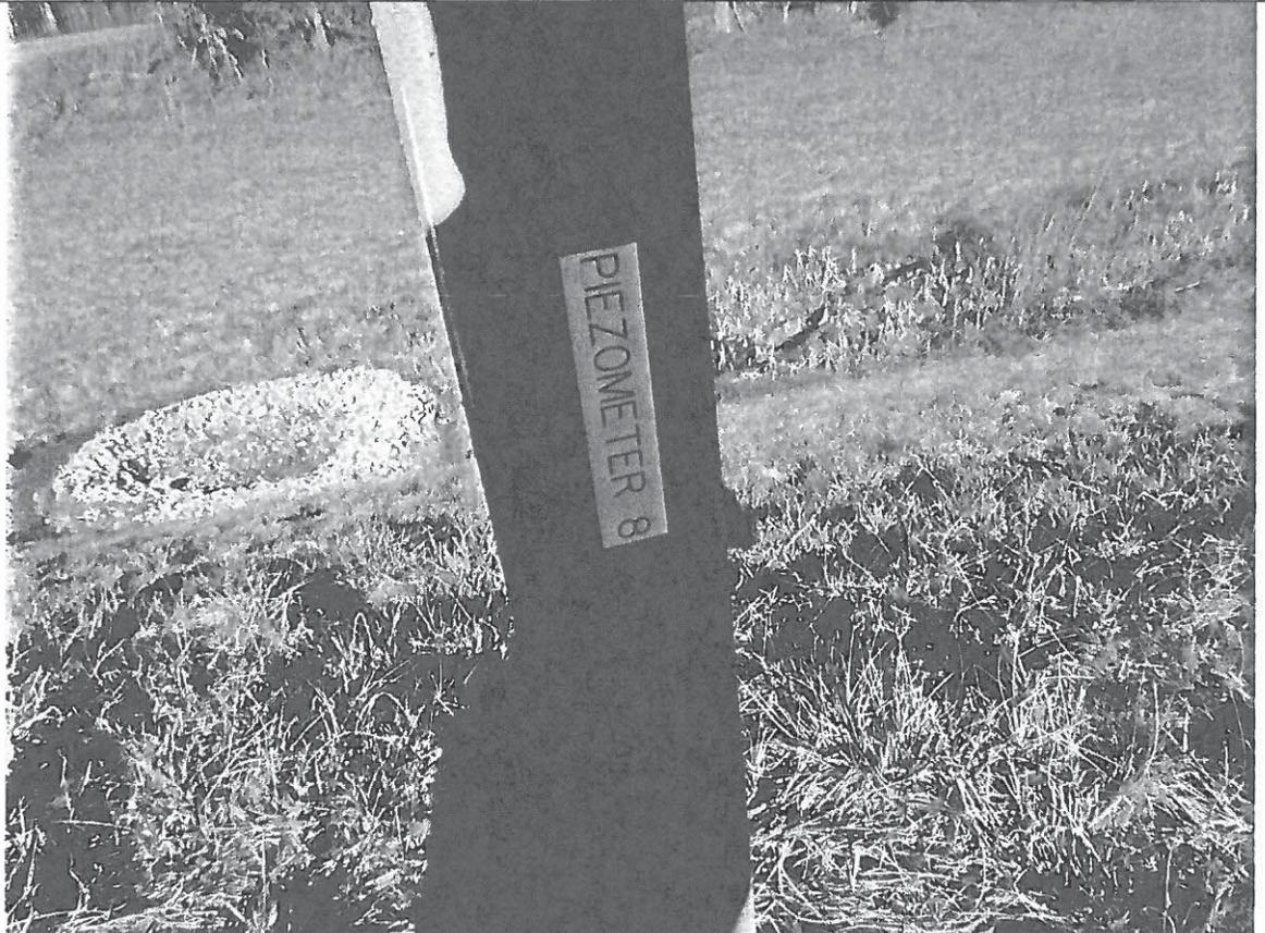
**Photo 10-** Piezometer 9 mislabeled as Piezometer 8. Rust is showing thru paint.
