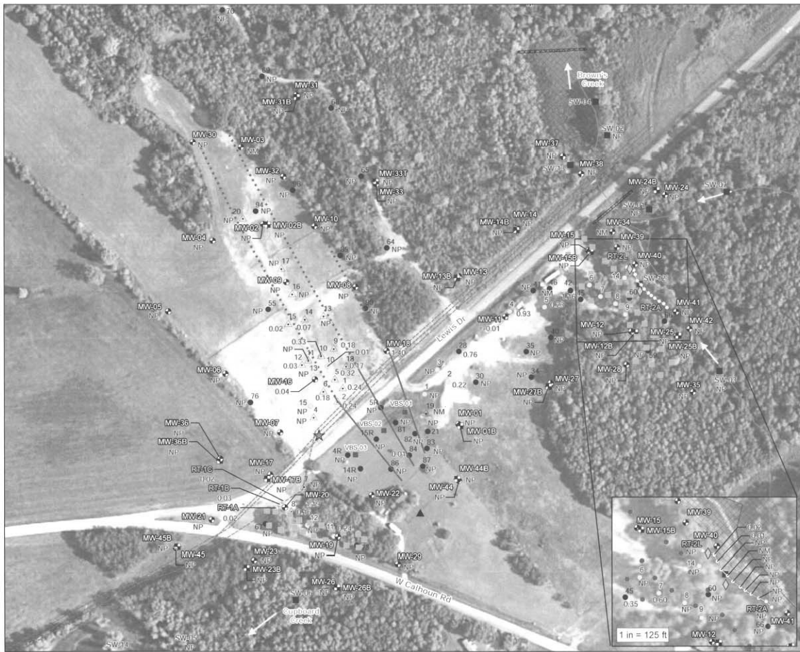
Figure 2. Product Thickness Map Lewis Drive Remediation, Belton, South Carolina Site ID #18593 "Kinder Morgan Belton Pipeline Release"
