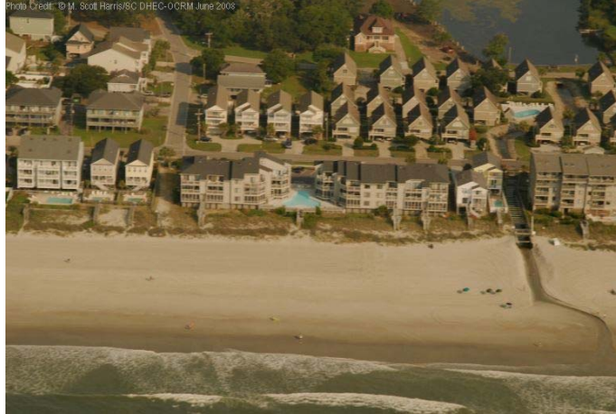
Figure 37. Aerial photograph of northern Surfside Beach. Notice the change in width of the upper beach due to renourishment (photo credit Scott Harris and DHEC, June 25, 2008).
