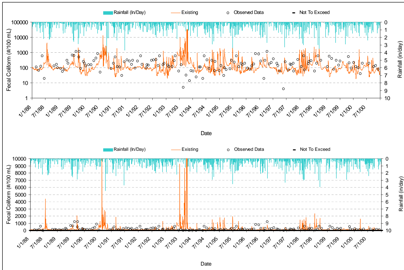
Figure D-5. Fecal coliform calibration at water quality station E-051
