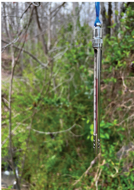
Hang the thermometer in the shade to measure air temperature first.
