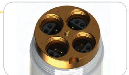
EXO1 sonde contains 4 universal sensor ports
