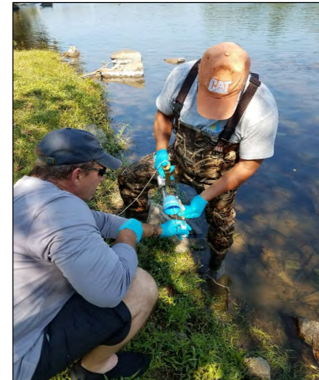
Use of Van Dorn Sampling Device (Typical)
