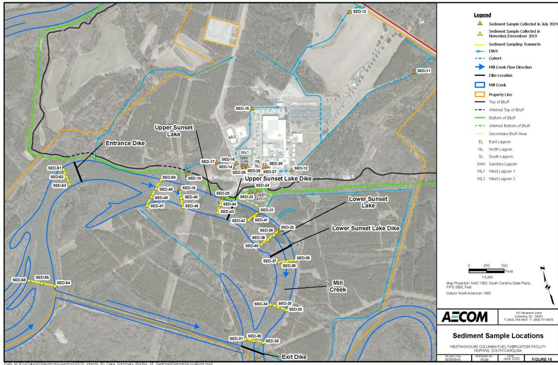
Mill Creek is a naturally meandering creek that was dammed to create Upper and Lower Sunset Lake, prior to the establishment of the Westinghouse Columbia site. A diversion canal was also created that redirected a majority of the water flow, limiting the volume of water in Upper and Lower Sunset Lake, and creating nearly stagnant conditions. This low flow of water through the Upper and Lower Sunset Lake, combined with the thick growth of trees and brush has created swamp like conditions.
