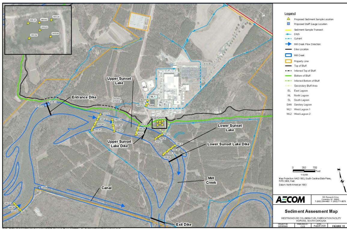
RI Phase II sediment samples were collected from the previous Phase I locations at deeper intervals, and at new locations to bound previously identified areas of elevated residual radioactivity.
