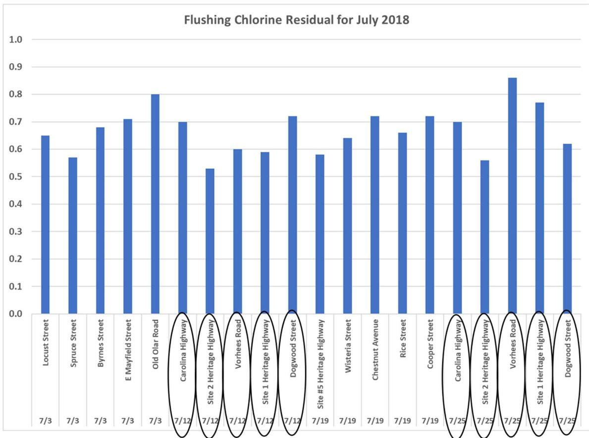
**FIGURE 16. Free chlorine residual at flushing sites (post flushing) during July 2018.**
