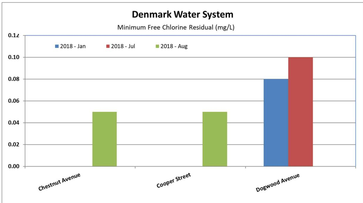
**FIGURE 15. Sampling events when free chlorine residual was < 0.20 mg/L at monitoring sites in 2018.**
