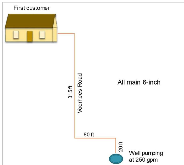
**FIGURE 8. West Voorhees piping arrangement and flow.**
