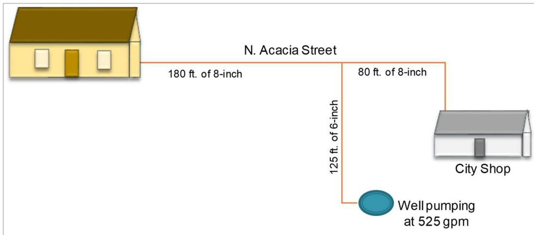
**FIGURE 10. Acacia piping arrangement and flow.**
