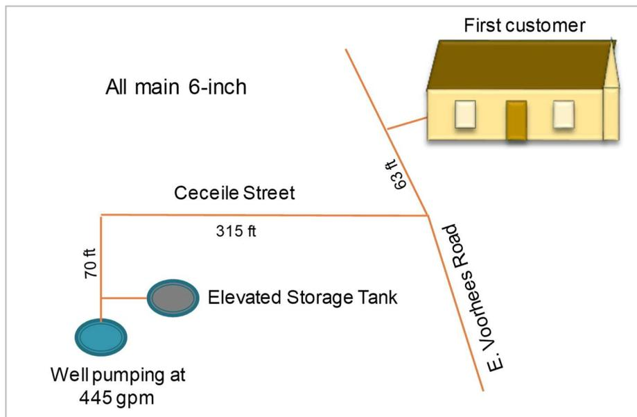
**FIGURE 9. East Voorhees piping arrangement and flow.**
