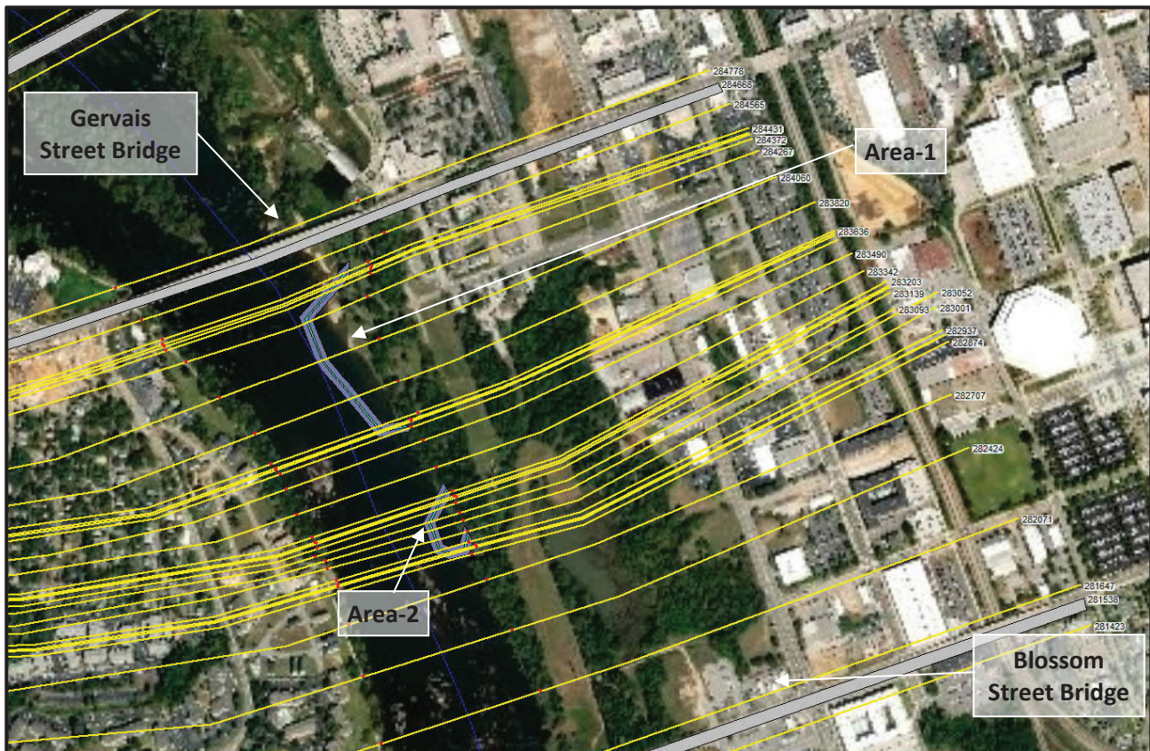
Figure 4: Corrected Effective HEC-RAS Model Schematic (Project Area)
