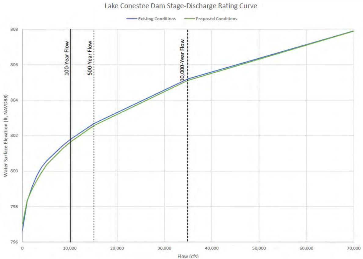
**FIGURE 17 LAKE CONESTEE DAM STAGE DISCHARGE RATING CURVE**
