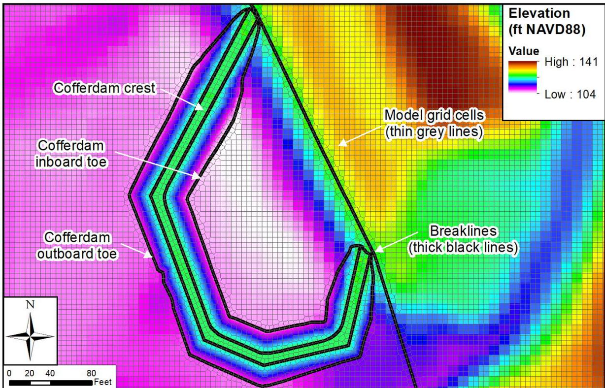
Figure 7: Proposed Area 2 Cofferdam Mesh Details
