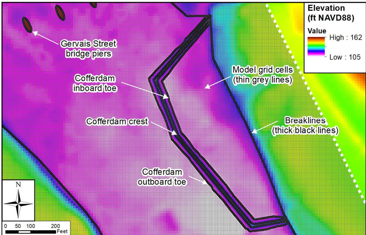
Figure 5: Proposed Area 1 Cofferdam Mesh Details
