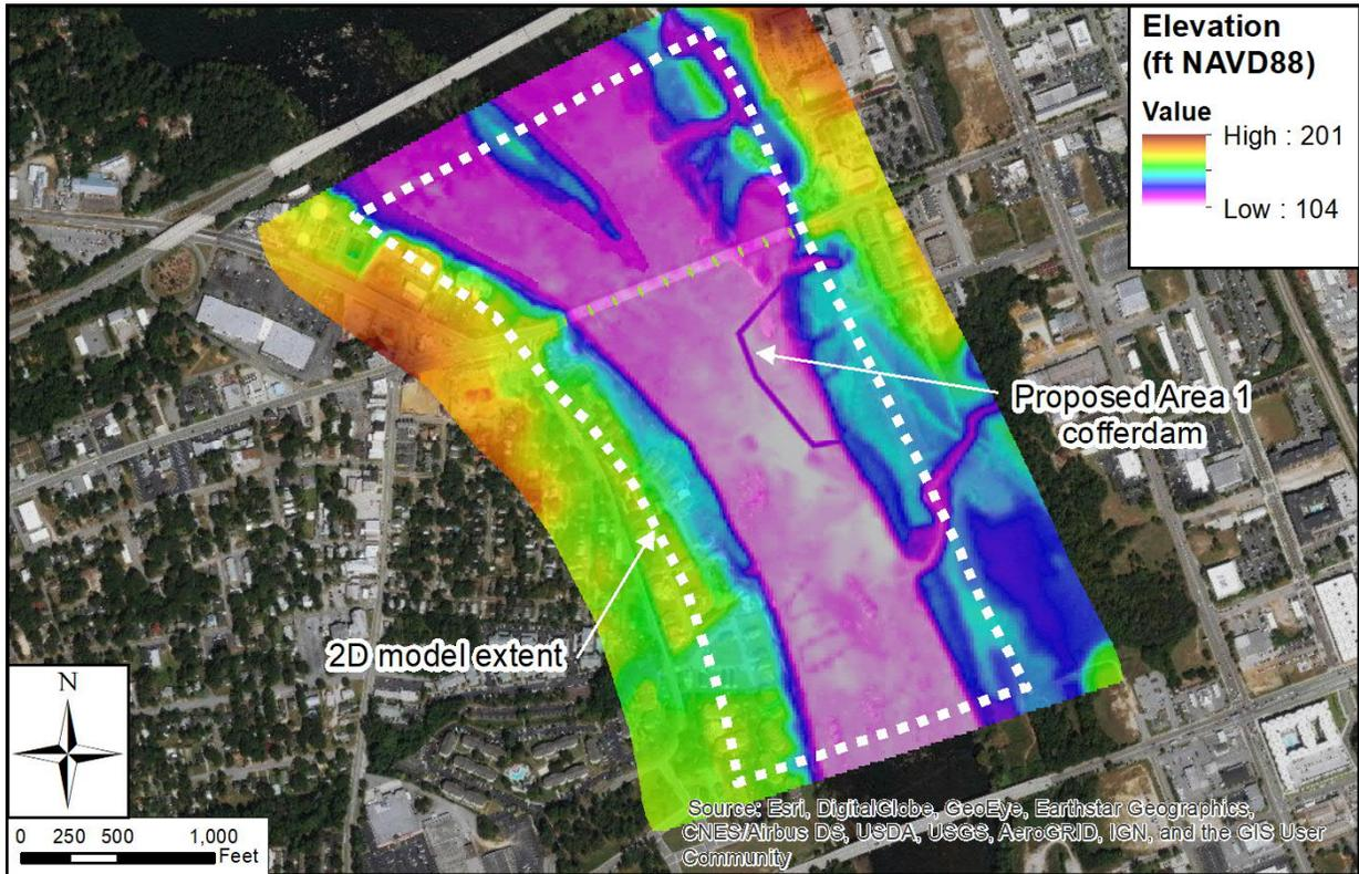
Figure 4: Proposed Area 1 Cofferdam Digital Elevation Model
