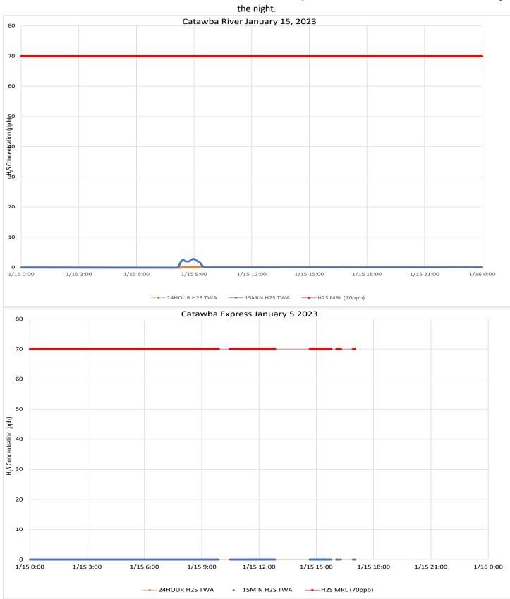
The Catawba Express monitor is offline due to a sample pump failure.
