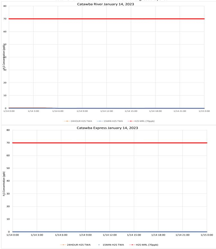
The Catawba Express monitor began having intermittent sample flow problems about 10AM, leading up to an indication of a sample pump failure. Summary data up to the time of the first sample air flow problem are valid.
