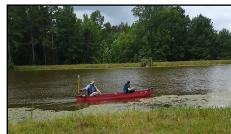
The canoe setup used for performing bathymetric surveys
