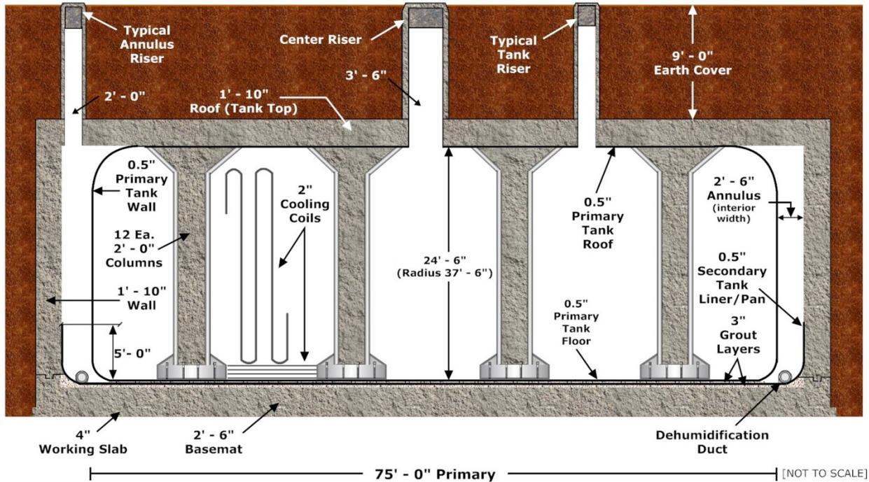
The Type I primary liner is made of 0.5-inch thick carbon steel. The liner wall is joined to the primary liner roof and floor with non-stress-relieved welded knuckle plates also made of carbon steel. The secondary liner is also made of 0.5-inch thick carbon steel. The top edge of the secondary liner has an L-shaped carbon steel stiffener lip that extends 6 inches perpendicularly inward from the liner edge with another 4-inch long section extending perpendicularly down from that edge. [W145367]
