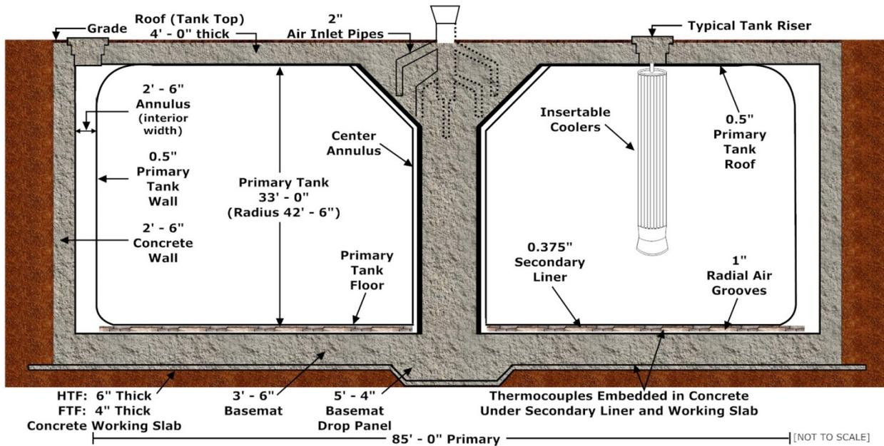
Figure 4.3-2: Typical Type IIIA Tank Cross-Section
