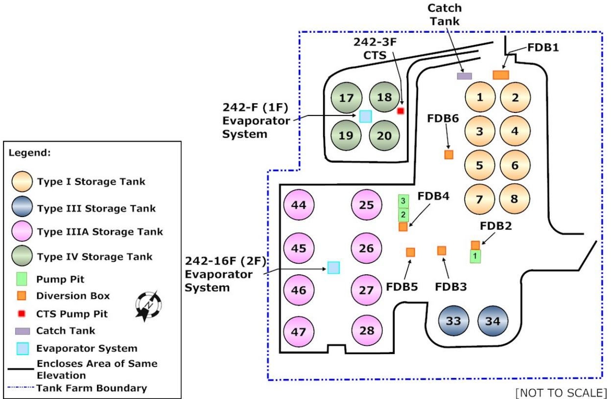
Figure 5.1-4: Layout of the H-Area Tank Farm
