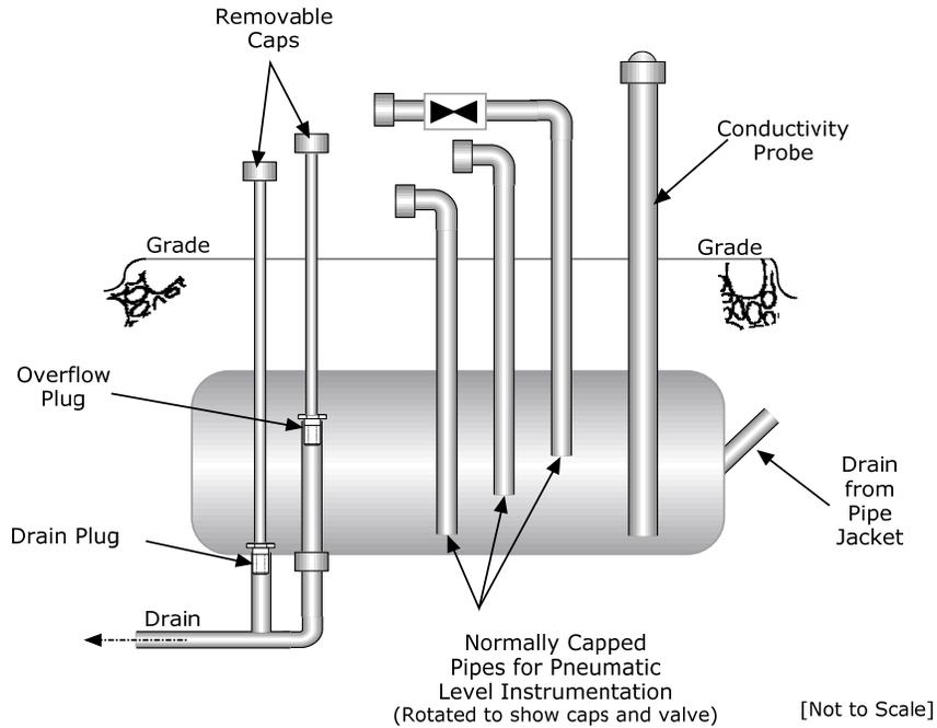
Figure 5.3-6: Typical Modified Leak Detection Box
