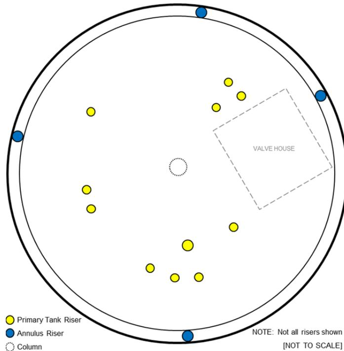
Figure 4.2-5: Typical Type II Tank Access Risers
