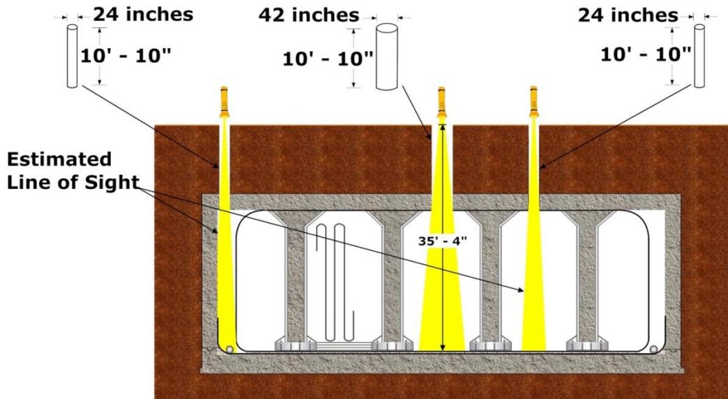
**NOTE: Risers may be impeded by installed equipment.**
