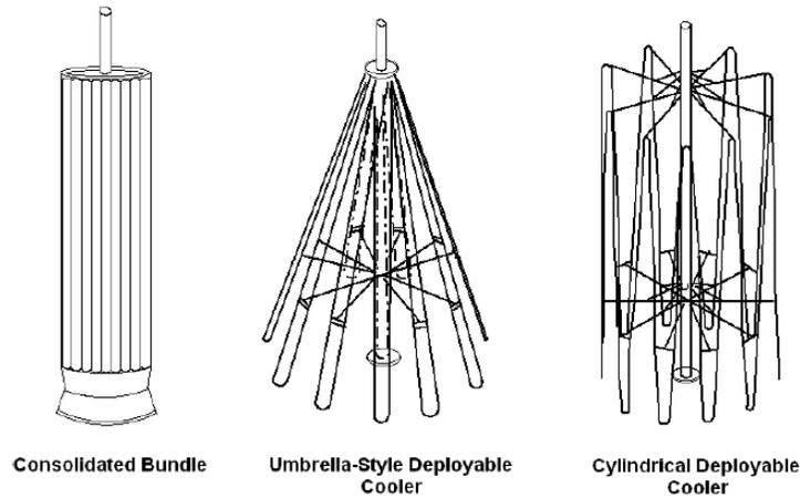
**Figure 4.3-5: Cooling Coils in a Type IIIA Tank**
