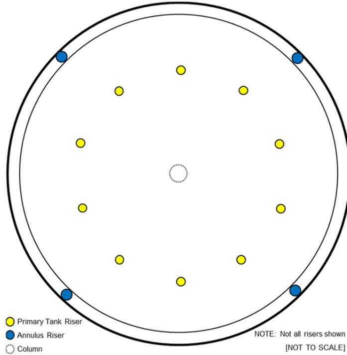
Figure 4.3-7: Typical Type IIIA Tank Riser Configuration
