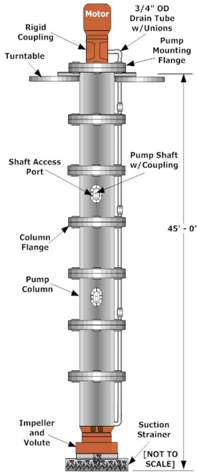
**Figure 7.1-2: Slurry Pump Turntable**
