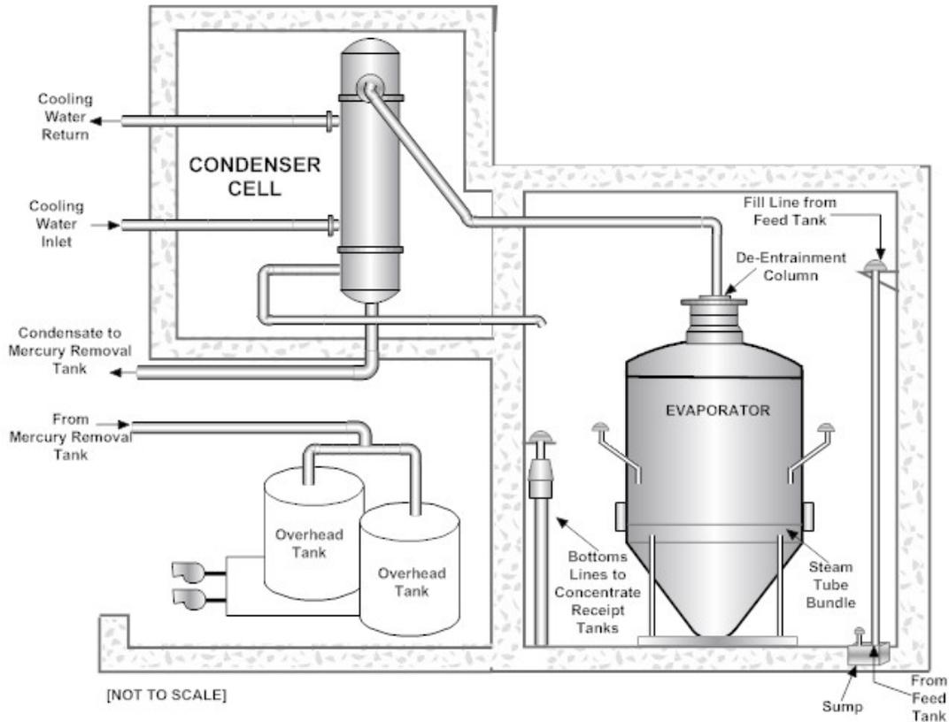
Note: Jumpers from the evaporator pot to the receipt tanks and from the feed tank to the condenser were not included to minimize the complexity of the figure.
