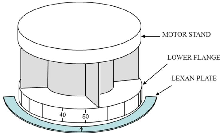
Note: The pump index is shown set to the 48° position
