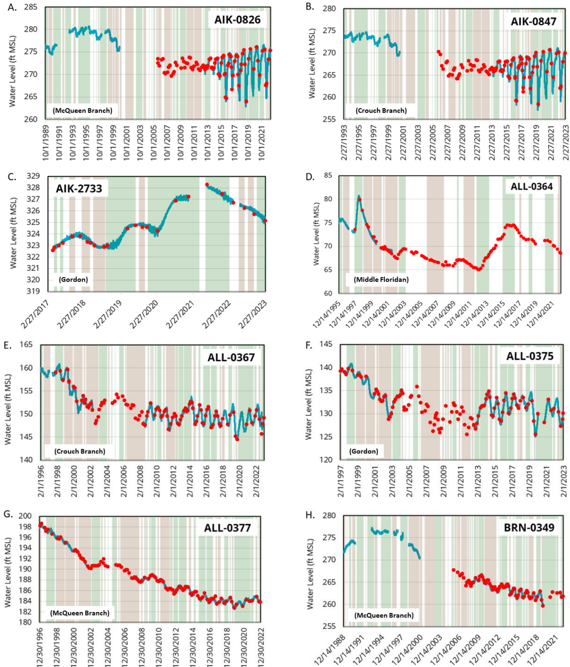
Figure 14. Water level plots from SCDNR monitoring wells in the Western Area. Water levels are in feet relative to sea level (MSL). The blue lines represent automatic data recordings and red dots represent manual water level measurements. The green background indicates wet periods, and the brown background indicates dry periods. http://hydrology.SCDNR.sc.gov/groundwater-data/ and https://www.drought.gov/states/south-carolina ; accessed March 31, 2023.
